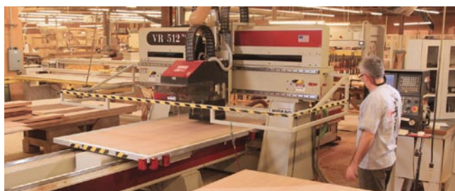
Above: among the CNC machines used at Zepsa is a Schelling saw and this Komo router. Left: by slicing horizontally on the Baker resaw, Zepsa can bookmatch thick lumber pieces. Below: Zepsa has the capability to lay up veneers in-house, using a custom Joos hot press.
