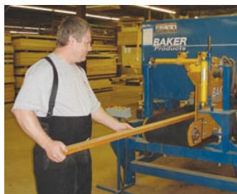
Above: among the CNC machines used at Zepsa is a Schelling saw and this Komo router. Left: by slicing horizontally on the Baker resaw, Zepsa can bookmatch thick lumber pieces. Below: Zepsa has the capability to lay up veneers in-house, using a custom Joos hot press.
